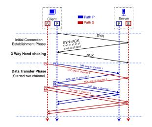
Fig. 4. Three-way handshaking between client and server and data transfer between them. Handshaking can go between any two pairs of interfaces. Here P is the primary path and S is one of the secondary or alternative paths.
