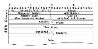
Fig. 5. Viscous packet header structure
